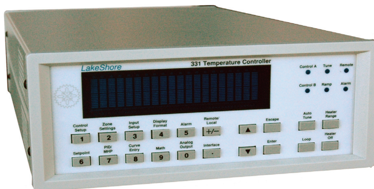
Figure 12.3h Lakeshore Controller Front Panel
