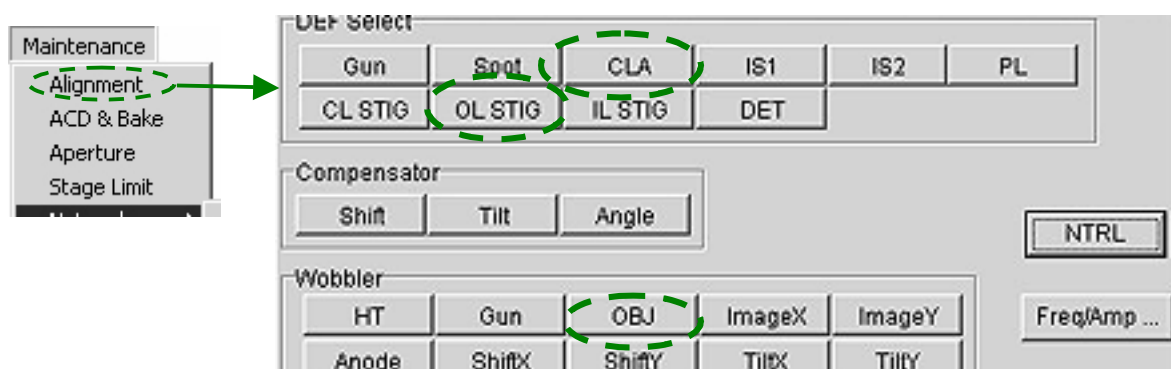
Fig. 5.39 Alignment Panel for Maintenance window (Observing low-magnification images)
