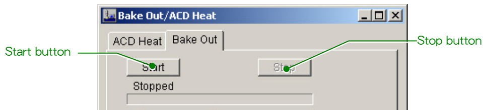
Fig. 6.22 Starting baking out (Bake Out/ACD Heat window)
