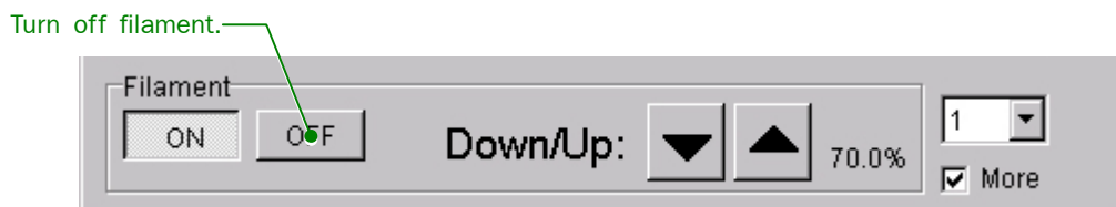
Fig. 5.16 High Voltage Control window(Turning off the filament)
